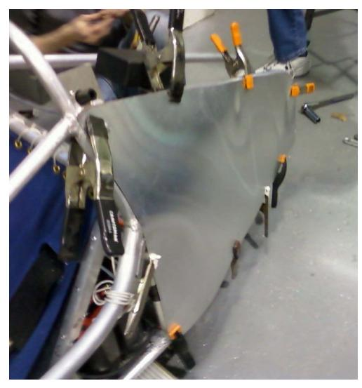
The 0.024 inch thick aluminum sheet was shaped for the rear and side panels, and each panel was clamped into place to verify the fit. The rear panels shown here, the battery cover panels, and the solar array will all be mounted with dzus fasteners. These fasteners will provide quick access to the drive system and batteries.
