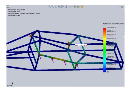
The selection of 6061 T1 Aluminum required an extensive ANSYS analysis of the frame and roll cage. The protection of the driver in the event of a frontal or side impact and roll-over were upmost in Zach's frame design analysis. Frontal and side impact ratings yielded a safety factor of 6 while the rollover safety factor yielded a safety factor of 14. The industry standard for a motorized vehicle is a safety factor of 5.
