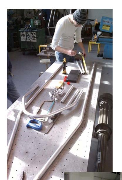
With the frame members verified by the mock-up, Zach began cutting and forming the aluminum tube on the assembly table. The basic frame material size was 1 inch OD, while the side impact members were 1-1/4 inch OD tubing.
