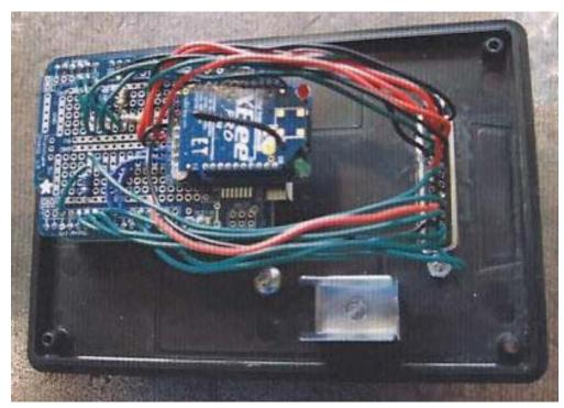
The in-vehicle instrumentation and telemetry box contained both an Arduino microcontroller board and an XBee transceiver. Therefore, information was hard-wired to an instrument box for the driver as well as being transmitted to the pits.
