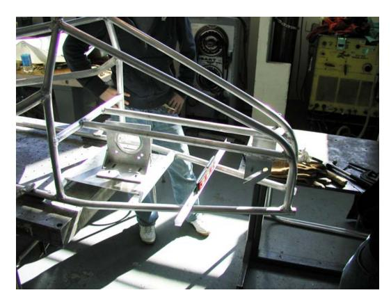
The tubes for the motor controller and the initial rear axel dropouts have now been welded in place. The mounting base for the motor mount bracket has also been welded in place across the base frame tubes. The level across the base frame tubes was used to correct for some minor bending which occurred during the welding process. The dropouts had to be perfectly level with the ground.
