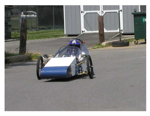
With only a minor tuning of the motor controller (a change in the ramp rate for acceleration), all of the electrical and mechanical systems were working perfectly. Obviously there was time out to paint the car and apply the vinyl lettering.
