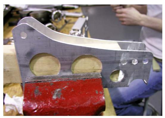
The A arm mounting brackets were fabricated from 6 x 2 in rectangular tubing. Initial mounting points were adjustable. The caster angle was established, and the mounting brackets were welded in place at the correct caster angle. Minor caster and chamber adjustments can still be made by turning the heim joints in or out.
