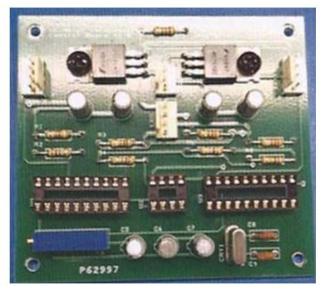
As for Joe's motor controller, after the boards were designed, Joe made full scale layout mock-ups to review the traces and to ensure that each component fit the footprint properly. Once the printed circuit boards arrived, the parts were soldered in place and the testing could continue. The upper picture shows the "Control Board", and the lower picture shows the "Power Board".
