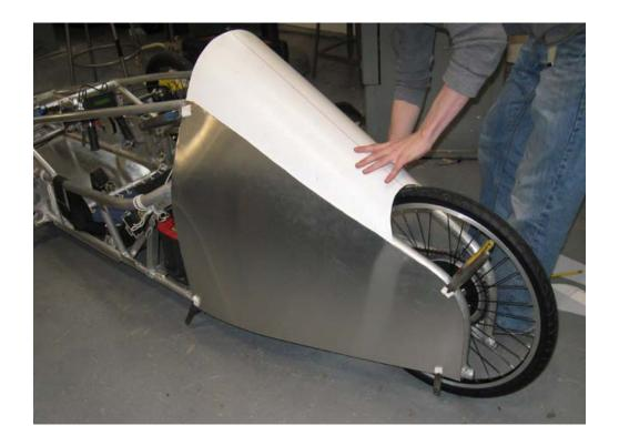
The Lexan polycarbonate cover (shown above with it's protective cover) is held in place in preparation for locating dzus fasteners for the rear side covers. The polycarbonate material was chosen for this rear cover area to insure that no interference would be created for the telemetry box mounted high in this area.
