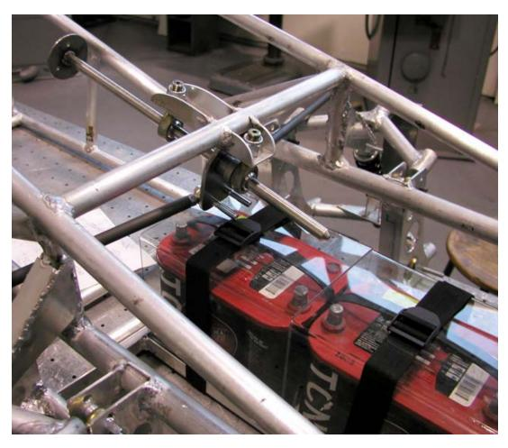
The steering column support bracket, the heim joint steering column supports, the pitman arm, and the tie rods were machined and welded into place. The original battery location can also be seen in this illustration. The battery location was later moved to the area behind the driver's seat in order to relocate the CG.
